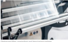
timised film unwinding and tensioning system
